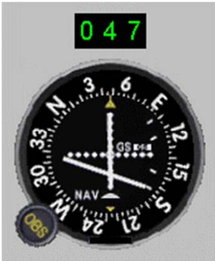
Aircraft above the glide path On the glide path http://www.navfltsm.addr.com/ils.htm
