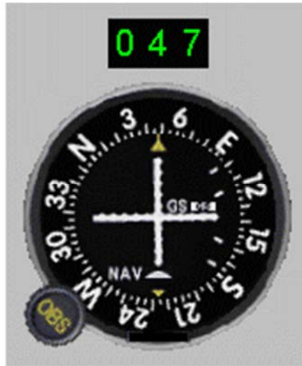
Aircraft above the glide path On the glide path http://www.navfltsm.addr.com/ils.htm
